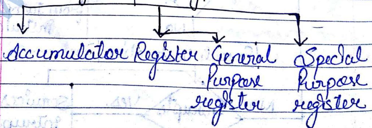
1- Accumulator Register :- In computer central processing unit (CPU) an accumulator register is a register which perform connection b/w general purpose register and special purpose register. Accumulator register perform intermediate b/w arithmetic and logical operations. This register is used to storing the results those produce by CPU. When the CPU will generates some results after the processing then all result will be stored in accumulator register.
